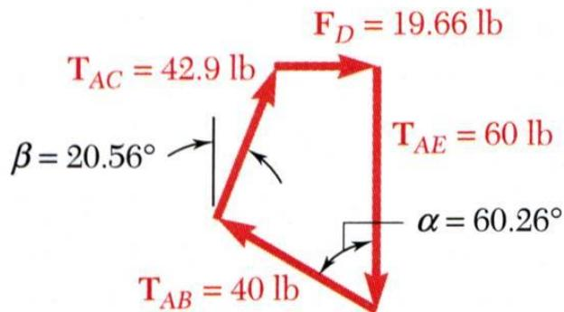
$$\begin{aligned}\vec{R} &= 0 \\ &= (-34.73 + 0.3512T_{AC} + F_D)\vec{i} \\ &\quad + (19.84 + 0.9363T_{AC} - 60)\vec{j}\end{aligned}$$
