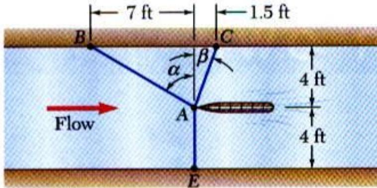
It is desired to determine the drag force at a given speed on a prototype sailboat hull. A model is placed in a test channel and three cables are used to align its bow on the channel centerline. For a given speed, the tension is 40 lb in cable  $AB$  and 60 lb in cable  $AE$ .
