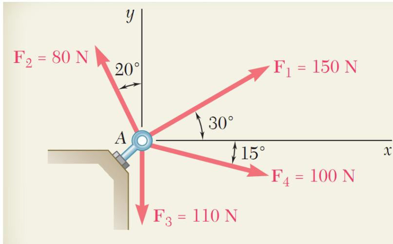
Four forces act on bolt A as shown. Determine the resultant of the force on the bolt.
