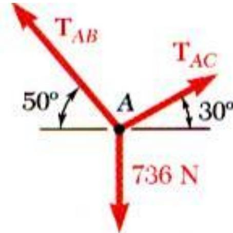
*Free-Body Diagram:* A sketch showing only the forces on the selected particle.
