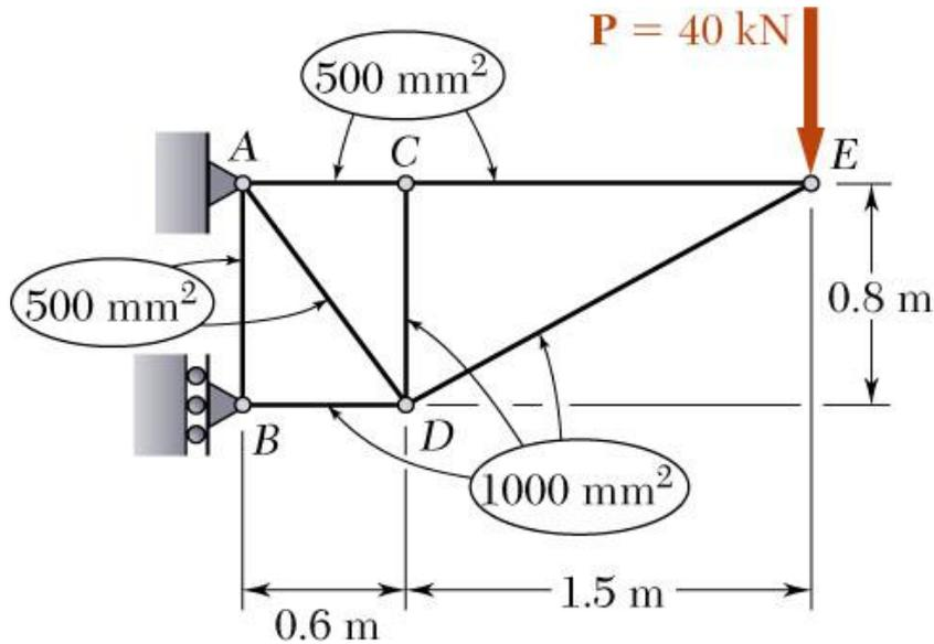
Members of the truss shown consist of sections of aluminum pipe with the cross-sectional areas indicated. Using  $E = 73 \text{ GPa}$ , determine the vertical deflection of the point  $E$  caused by the load  $P$ .
