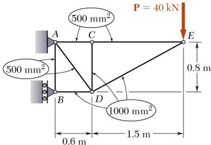
Members of the truss shown consist of sections of aluminum pipe with the cross-sectional areas indicated. Using  $E = 73 \text{ GPa}$ , determine the vertical deflection of the joint  $C$  caused by the load  $P$ .
