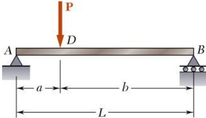
Taking into account only the normal stresses due to bending, determine the vertical displacement at cross-section  $D$  of the beam for the loading shown.
