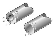
2. The tubular drive shaft for the propeller of a hover-craft is 6 m long. If the motor delivers 4 MW of power to the shaft when the propellers rotate at 25 rad/s, determine the required inner diameter of the shaft if the outer diameter is 250 mm. What is the angle of twist of the shaft when it is operating? Take [7 ] = 90 MPa and G = 75 GPa.【图示气垫式运输机的推进驱动轴为一外直径为 250 mm、长 6 m 的空心轴,在功率为 4 MW 的推进电机驱动下以 25 rad/s 旋转,若该轴的许用切应力为[7 ] = 90 MPa,剪切模量 G = 75 GPa,试求该轴最小所需内直径,并求对应的扭转角。】
