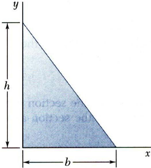
Determine the product of inertia of the right triangle (a) with respect to the  $x$  and  $y$  axes and (b) with respect to centroidal axes parallel to the  $x$  and  $y$  axes.
