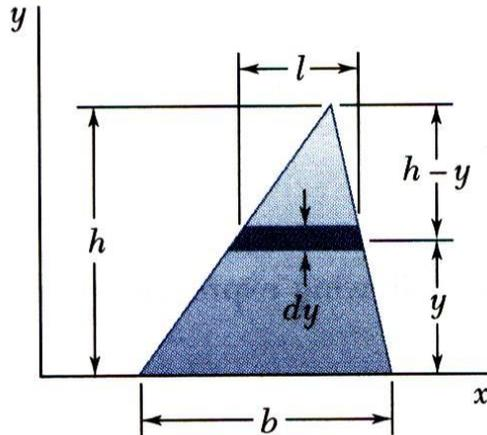
Determine the moments of inertia of a triangle with respect to its base.
