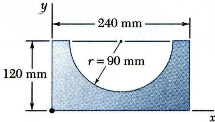
Determine the moments of inertia of the shaded area with respect to the  $x$  axis.
