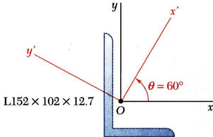
The moments and product of inertia with respect to the  $x$  and  $y$  axes are  $I_x = 7.24 \times 10^6 \text{ mm}^4$ ,  $I_y = 2.61 \times 10^6 \text{ mm}^4$ , and  $I_{xy} = -2.54 \times 10^6 \text{ mm}^4$ .
