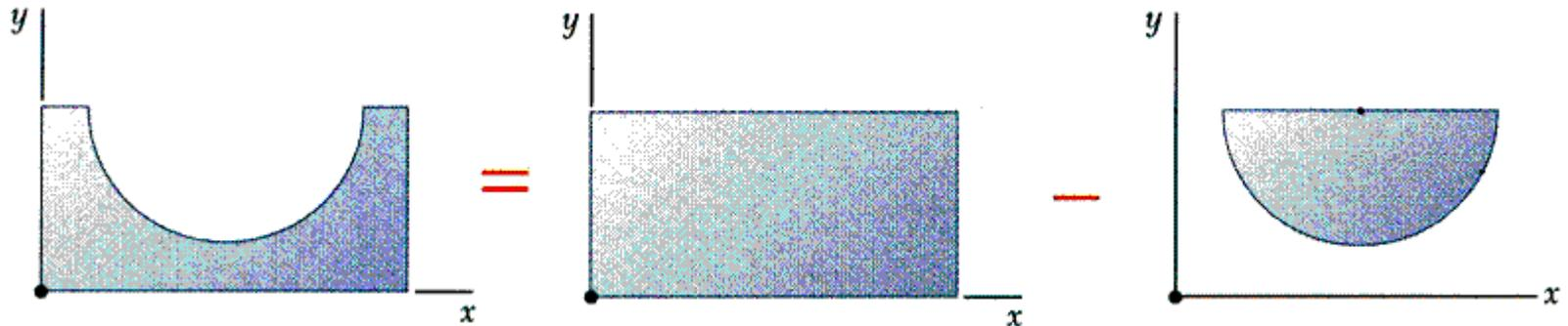
$$I_x = 138.2 \times 10^6 \text{ mm}^4 - 92.3 \times 10^6 \text{ mm}^4$$
