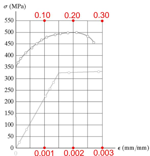
3. The stress-strain diagram for a polyester resin is given in the figure. If the rigid beam  $AC$  is supported by a strut  $AB$  and post  $CD$  made from this material, determine the largest load  $P$  that can be applied to the beam before  $AB$  or  $CD$  ruptures. The diameter of the strut is 12 mm and the diameter of the post is 40 mm. 【聚酯树脂的拉压应力应变曲线如右图所示，左图中的钢梁  $AC$  由该材料制成的杆  $AB$ （直径 12 mm）和  $CD$ （直径 40 mm）支撑，试求  $AB$  或  $CD$  断裂前钢梁所能承受的最大荷载  $P$ 。】
