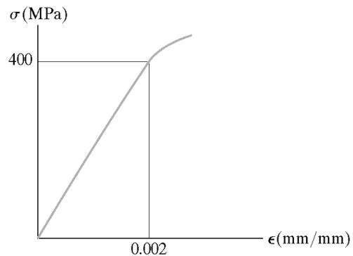
2. The stress-strain diagram for a steel bar is shown in the figure. Determine approximately the modulus of elasticity, the proportional limit, the ultimate stress, the fracture stress and the modulus of resilience. If the bar is loaded until it is stressed to 450 MPa, determine the amount of elastic strain recovery and the permanent set of strain in the bar when it is unloaded. 【一钢杆的拉伸应力应变曲线如图所示，试求其弹性模量、比例极限、强度极限、断裂应力和回弹模量（弹性应变能密度）；若在加载到应力为 450 MPa 时卸载，试求可以恢复的弹性应变和不可恢复的永久塑性应变。】
