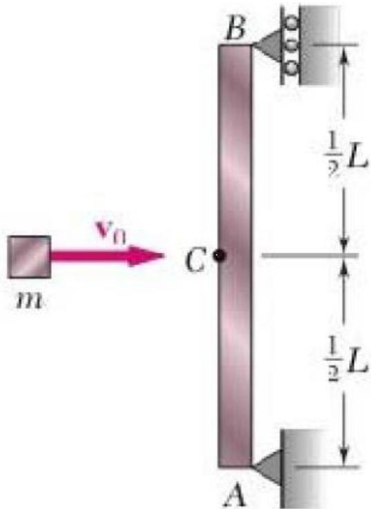
**Horizontal Impact:** A block of mass  $m$  moving with a velocity  $v_0$  hits squarely the prismatic member  $AB$  at its midpoint  $C$ . Determine (a) the equivalent static load  $P$ , (b) the maximum stress  $\sigma_{max}$  in the member, and (c) the maximum deflection  $\Delta_{max}$  at  $C$ .
