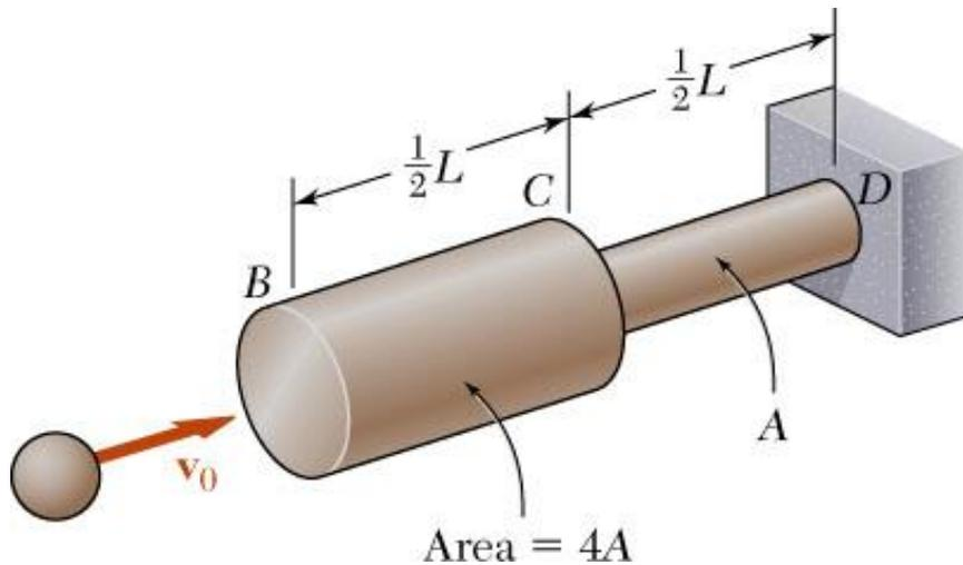
**Horizontal Impact:** Body of mass  $m$  with velocity  $v_0$  hits the end of the nonuniform rod  $BCD$ . Knowing that the diameter of the portion  $BC$  is twice the diameter of portion  $CD$ , determine the maximum value of the normal stress in the rod.
