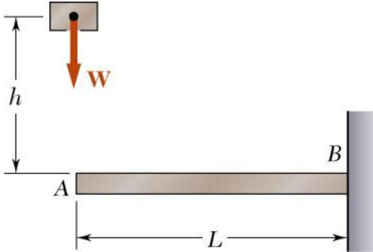
**Vertical Impact:** A block of weight  $W$  is dropped from a height  $h$  onto the free end of the cantilever beam. Determine the maximum value of the stresses in the beam.
