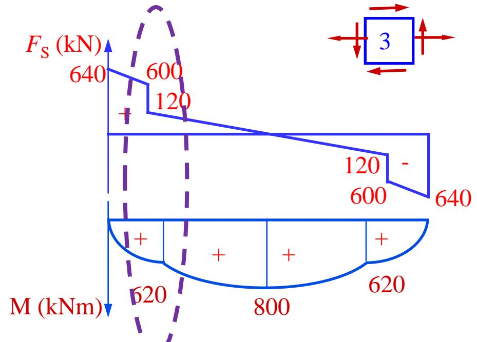
$$\sigma = \frac{My}{I_z} = \frac{620 \times 10^3 \times 400 \times 10^{-3}}{2.126 \times 10^{-3}} = 116.7 \text{ MPa} < [\sigma]$$
