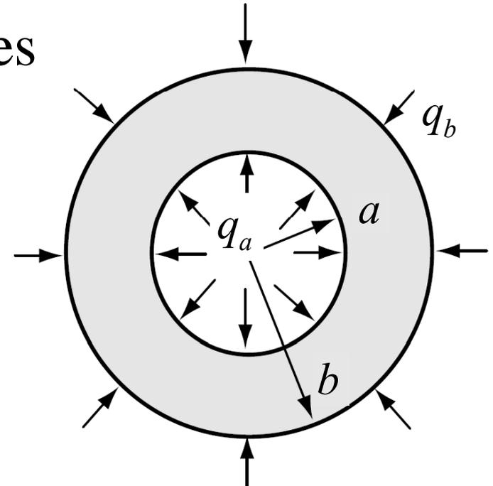
$$\Rightarrow \begin{cases} \sigma_R = \lambda \left( \frac{\partial u_R}{\partial R} + \frac{2u_R}{R} \right) + 2G \frac{\partial u_R}{\partial R} = \lambda \left( A - \frac{2B}{R^3} + 2A + \frac{2B}{R^3} \right) + 2G \left( A - \frac{2B}{R^3} \right) \\ \sigma_\varphi = \sigma_\theta = \lambda \left( \frac{\partial u_R}{\partial R} + \frac{2u_R}{R} \right) + 2G \frac{u_R}{R} = \lambda \left( A - \frac{2B}{R^3} + 2A + 2 \frac{B}{R^3} \right) + 2G \left( A + \frac{B}{R^3} \right) \end{cases}$$
