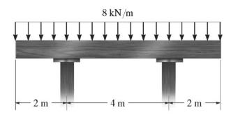
2. The beam is subjected to a uniform load w. Determine the placement a of the supports so that the shearing stress in the beam is as small as possible. What is this stress?【试求当图示梁中弯曲切 应力的最大绝对值取最小值时的支撑位置 a, 并求对应的最大弯曲切应力。】
