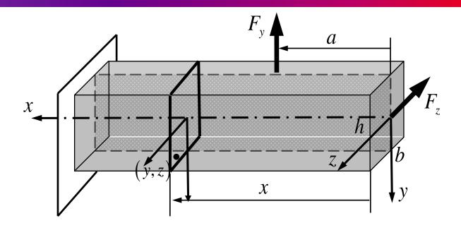
$$M_{z} = F_{y}(x-a), \ \sigma'_{x} = \frac{M_{z}y}{I_{z}}, \ a \le x \le L$$
