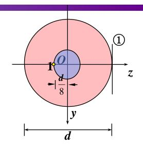
• Due to axial symmetry, only one neutral axis is necessary to determine the radius of the core area:
