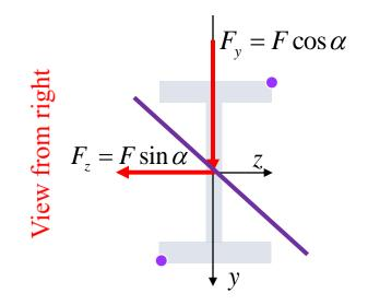
**Remark**: The fact that the neutral axis is not necessarily perpendicular to the resultant moment can greatly affect the stresses in a beam, especially if the ratio of the principal moments of inertia is very large. Under these conditions the stresses in the beam are very sensitive to slight changes in the direction of the load and to irregularities in the alignment of the beam itself.
