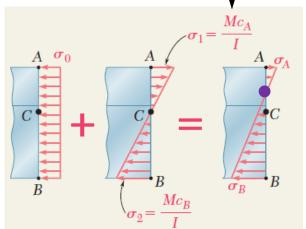
• Determine an equivalent centric and bending loads.
