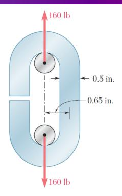
An open-link chain is obtained by bending low-carbon steel rods into the shape shown. For 160 lb load, determine (a) maximum tensile and compressive stresses, (b) distance between section centroid and neutral axis
