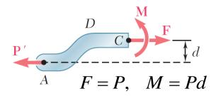
• Stress due to eccentric loading found by superposing the uniform stress due to a centric load and linear stress distribution due a pure bending moment
