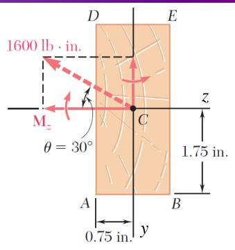
• Resolve the couple vector into components and calculate the corresponding maximum stresses.
