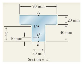
The largest allowable stresses for the cast iron link are 30 MPa in tension and 120 MPa in compression. Determine the largest force *P* which can be applied to the link and the neutral axis.
