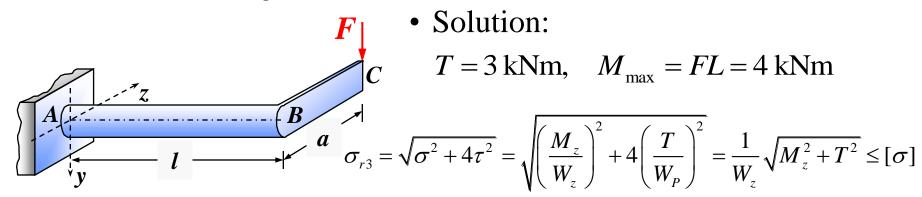
$$T = 3 \text{ kNm}, \quad M_{\text{max}} = FL = 4 \text{ kNm}$$
