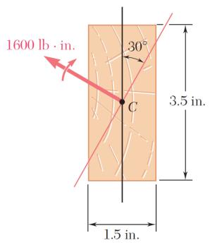
A 1600 lb-in couple is applied to a rectangular wooden beam in a plane forming an angle of 30 deg. with the vertical. Determine (a) the maximum stress in the beam, (b) the angle that the neutral axis forms with the horizontal plane.
