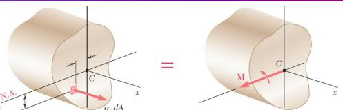
Wish to determine the conditions under which the neutral axis of a cross section of arbitrary shape coincides with the axis of the moment as shown.
