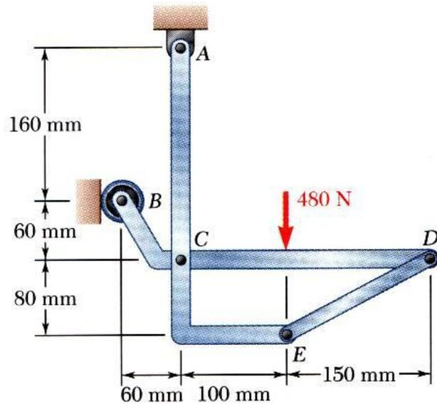
Members  $ACE$  and  $BCD$  are connected by a pin at  $C$  and by the link  $DE$ . For the loading shown, determine the force in link  $DE$  and the components of the force exerted at  $C$  on member  $BCD$ .
