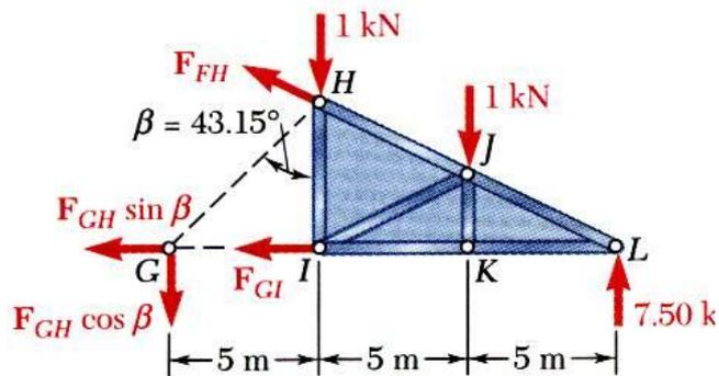
$$\tan \beta = \frac{GI}{HI} = \frac{5 \text{ m}}{\frac{2}{3}(8 \text{ m})} = 0.9375 \quad \beta = 43.15^\circ$$
