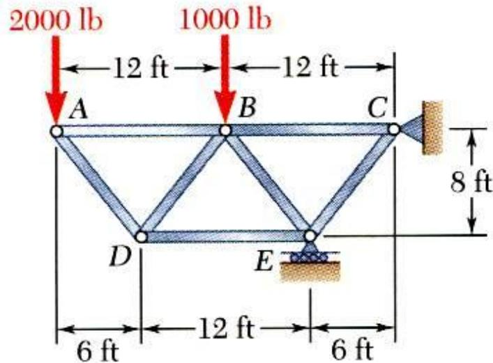
Using the method of joints, determine the force in each member of the truss.
