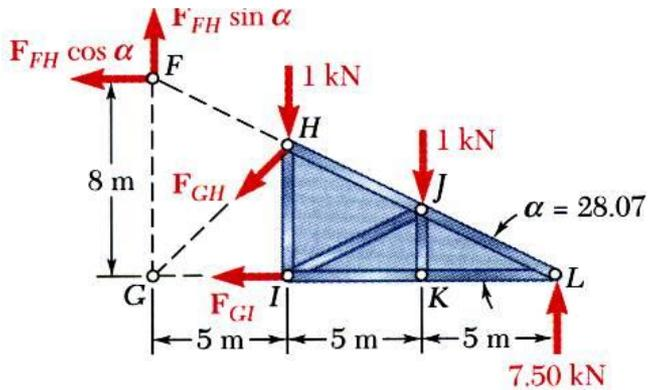
$$\tan \alpha = \frac{FG}{GL} = \frac{8 \text{ m}}{15 \text{ m}} = 0.5333 \quad \alpha = 28.07^\circ$$
