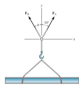
2. Determine the magnitude of F1 and its direction  $\theta$  so that the resultant force is directed vertically upward and has a magnitude of 800 N. 【如图所示,试求产生 竖直向上 800 N 的合力所需的  $\mathbf{F}_1$  的大小和方向( $\theta$  角)。】
