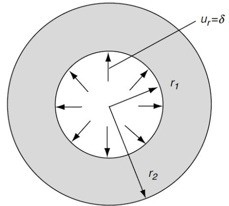
2. In class, we solved the problem of a thick-walled cylinder subjected to a uniform pressure on both the inner and outer boundary. Resolve this problem by replacing the traction boundary condition on the outer radius  $r_2$  with a zero-displacement condition, i.e.  $u_r(r_2) = 0$ .
