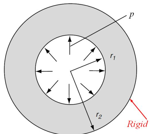
3. A long composite cylinder is subjected to the external pressure loading as shown. Assuming idealized perfect bonding between the two materials, i.e. the normal stress and displacement will be continuous across the interface  $r = r_1$ . Under these conditions, determine the stress and displacement fields in each material.
