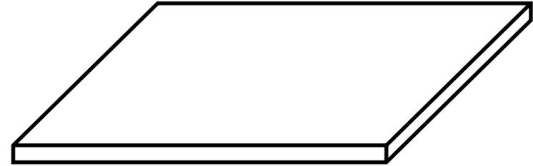
Plates: two dimensions are far greater than the third. No curvature exists in the median plane of the plate.
